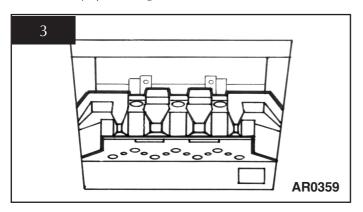
6.2 Locate the rear panel against the spacer brackets and slide down so that it locates on the ledge of the flame baffle. See diagram 4.
