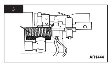
3.3 The pilot unit can now be removed by undoing the two screws. See diagram 6.
