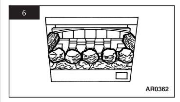
6.5 Place four of the loose round coals behind the first row so that they sit on the fingers, the two outer ones should touch the rectangular coals. See diagram 7.
