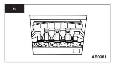
4.4 Place five of the loose round coals on the frint coal so that they lean against the flame baffle, in between the fingers. Place the two rectangular against the reflector panels, one either side, behind the front row of loose coals. See diagram 7.
