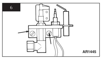
3.7 Reassemble in reverse order, do not overtighten. NOTE: SPECIAL CARE SHOULD BE TAKEN WHEN REPLACING THE THERMOCOUPLE TO THE BACK OF THE GAS VALVE TO ENSURE THAT THE SENOR WIRES FOR THE GAZCO FLUE SURE SYSTEM ARE NOT DISCONNECTED.
