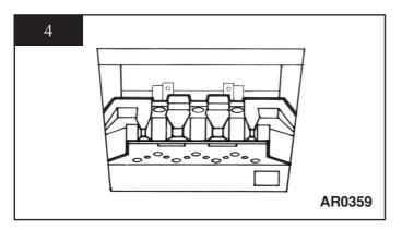
4.2 Locate the rear panel against the spacer brackets and slide down so that it locates on the ledge of the flame baffle. See diagram 5.
