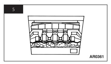
6.4 Place five of the loose round coals on the front coal so they lean against the flame baffle, in between the fingers. Place the two rectangular coals against the reflector panels, one either side, behind the front row of loose coals. See diagram 6.
