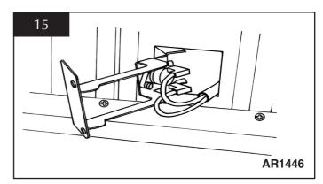
9.3 Refit the new sensor ensuring that the plastic spacers are located between the bracket and the sensor. Refit the leads. See diagram 16.
