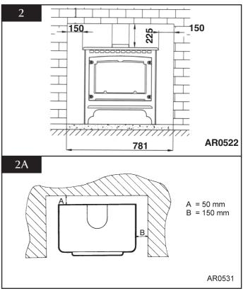
In a non-combustible recess attention must be given to allowing adequate clearance at the sides and rear of the stove, so that a spillage test can be performed, and the controls reached.
