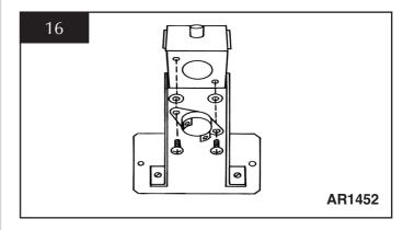
9.4 Feed the cable back through the hole as you replace the bracket. When the bracket is located correctly it will sit flush with the back panel without force being required. If not positioned correctly the bracket will sit at an angle. See diagram 17.
