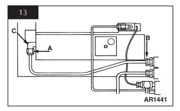
8.3 Reassemble in reverse order, the injector must **NOT** be tightened into the burner but be allowed to float to enable it to line up with the pipe. Turn on the gas supply and check for leaks.
