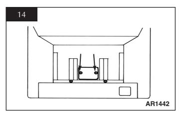
9.2 Disconnect the two sender wires. Undo the two taptite screws and remove the sensor and the two plastic spacers. See diagram 15.
