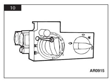
6.4 To release the right hand side of the control cover insert the narrow blade screwdriver into the slot shown in diagram 11, lever it gently and pull from the right hand side at the same time. The cover will now come off, there is a small cylindrical metal spacer inside the cover, this must be kept and replaced on the fixing screw during re-assembly.
