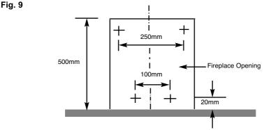
Fit the wallplugs provided and screw the fixing eyes securely into the rear of the fire opening.
