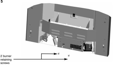
e) The base of the burner unit can now be lifted, lift the two retaining tabs on the burner brackets from the back of the firebox, allowing the burner to be removed. See fig. 6 below
