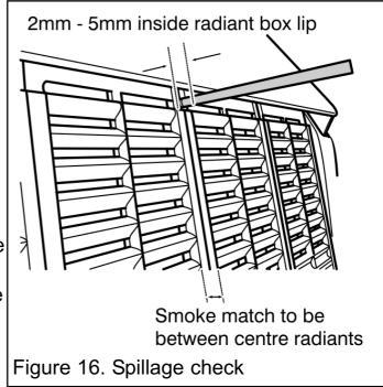
in the closed position (see section 6.6), reopen the restrictor, reseal the appliance and retest. If smoke is still not drawn into the appliance disconnect the appliance and seek expert advice
