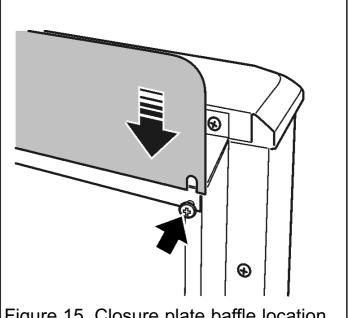
Figure 15. Closure plate baffle location
