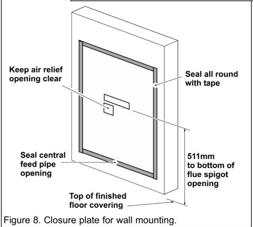
plate and observe the smoke. If there is a definite flow continue with the installation. If not check the fitting of the closure plate. The fireplace flue pull check described in section 5.2 should have confirmed that the fireplace itself is satisfactory.
