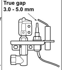
Figure 5. Pilot spark gap
