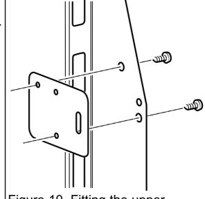
Figure 10. Fitting the upper extension brackets
