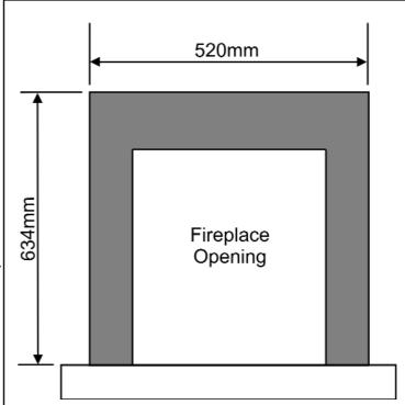
Figure 3. Area to be free of combustible cladding
