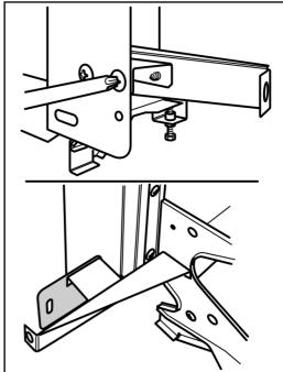
Figure 9. Fitting the lower extension brackets.
