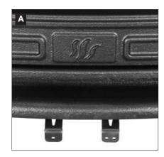
A Pull the secondary air slider (marked with a double hole) fully forward and open the primary air slider (marked with a single hole) fully by pulling the lever forward.
