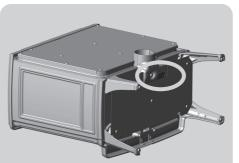
The stove incorporates a knock out destructive panel (circled) that can be removed if extra airflow is required for safe combustion.
