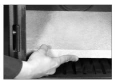
• Remove the internal baffle plate
