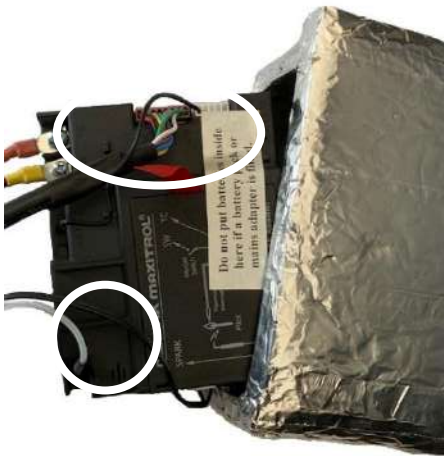
Picture 2 – Showing receiver unit being fitted into the Heat shield pocket – be careful not to pull any wires out of their multi-plug sockets as shown in the white circles
