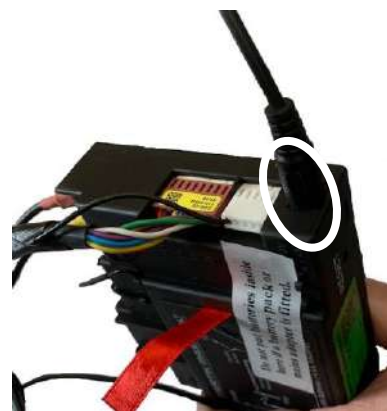
Pictures shows receiver unit with the Battery lead jack plug fitted – see white circle
