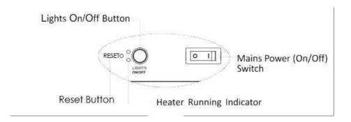
NOTE: The manual buttons control basic functions, not a full range of controls. Use the remote hand set to carry out all functions.
