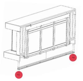
**18)** Install the bottom panel onto the underside to the surround with the four surround screws left over.
