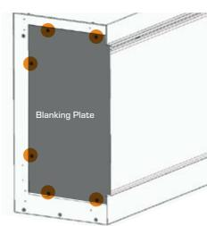
For a three-sided installation, secure the small and large trims on both ends of the appliance in line with the corresponding holes of the firebox. Secure into position with the 12 supplied firebox screws, six on each side.
