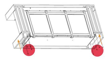
17) Underneath the appliance, with the surround screws, screw up through the bottom surround and into the legs of the surround top section and up through the floating shelf brackets on the appliance the top section.
