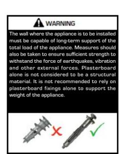
Check regularly for security of wall fixings as appropriate. Also check security of supply cable and connections. If the supply cable becomes damaged, it must be replaced by a service agent or competent person, such as a qualified electrician.
