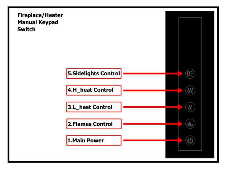
The upper segment of the control panel, (1), is the **Main Power** button. As the name infers, the Main Power button controls the overall power to the fireplace/heater unit. Pressing the button once turns power on to the entire unit, and pressing the button again will turn power off to the entire unit. If you find that none of the other buttons appear to work, check to make sure that Main Power is turned on to the unit.
