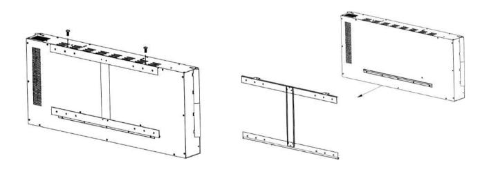
Step 2: Choose a solid and plain wall. Position the mounting bracket where the appliance is to be installed on the wall and ensure that the bracket is level. Using a pen mark the 4 holes through the 4 holes on the mounting bracket as shown below (Figure 2)
