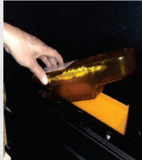
2. Lift water tank out of inset
