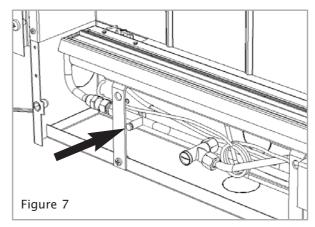
This will be dirt and debris, kinked or inadequate size pipes, restriction in a fitting, shut off elbow not fully open or solder flashing across a joint. Identify the cause of the restriction and rectify. Switch the fire off, disconnect the pressure gauge and refit the test nipple screw. Light the fire and check for gas soundness.
