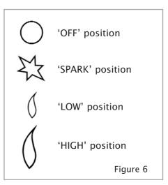
To achieve the HIGH setting, push the control knob in slightly and continue turning anti-clockwise to the high position. The main burner should light after a few seconds. To decrease the setting to LOW, turn the control knob clockwise to the low setting.
