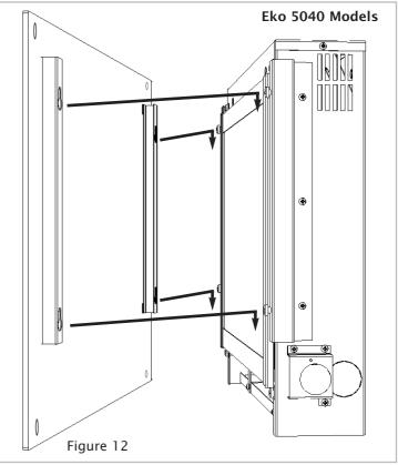
To fit the decorative corner columns, ensure the main glass facia is mounted in position. Remove any transit tape and unscrew the front clamping disc and remove.
