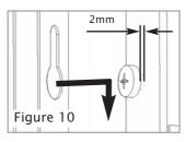
ate a 2mm gap (shown in figure 10). Simply hang the facia panel onto the outer casing (figure 12) ensuring that the corresponding keyhole shaped holes engage the screwheads fully.
