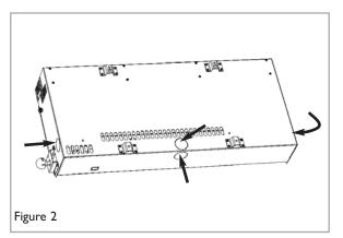
grommet supplied. A small incision can now be made in the rubber to slip snugly around the outside of the supply pipe and sleeving.
