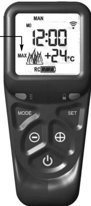
Fig. 3 - "MAX" & large flame symbol displayed
