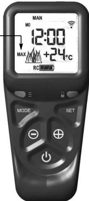
Fig. 35 - "MAX" & large flame symbol displayed
