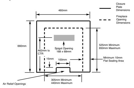
Apply a smoke match to the flue spigot opening in the closure plate and observe the smoke. If there is a definite flow into the opening then proceed with the installation. If there is not a definite flow into the opening, pre-heat the chimney for about two minutes and retest for flow. If there still is no definite flow into the opening, the chimney may require attention. DO NOT FIT THE FIRE-SEEK EXPERT ADVICE.
