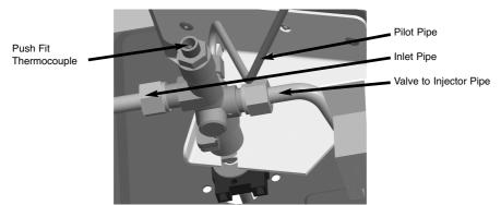
d) Remove the valve retaining nut as shown below and disconnect the wires to the microswitch as shown below in Fig. 18
