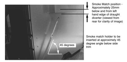
If there is an extractor fan fitted in a joining room, then the spillage test must be repeated with the fan switched on and running at maximum speed. All interconnecting doors must be opened in accordance with the latest issue of BS 5440.
