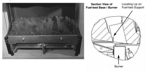
b) Fit coal "A" onto the fuelbed base in the position as shown below in Fig. 2. The coal form has the individual placement letters stamped on the bottom face.
