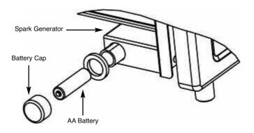
IN THE EVENT OF THE FIRE FAILING TO LIGHT, PLEASE VISUALLY CHECK FOR SPARKING AT THE IGNITION ELECTRODE ON THE PILOT. IF NO SPARK IS PRESENT PLEASE REPLACE THE BATTERY AS DETAILED ABOVE. SERVICE CALLS THAT ARE A DIRECT RESULT OF FLAT BATTERIES WILL BE CHARGED FOR BY THE MANUFACTURER AS THE BATTERY IN THE FIRE IS A CONSUMABLE ITEM THAT WILL REQUIRE ROUTINE REPLACEMENT.
