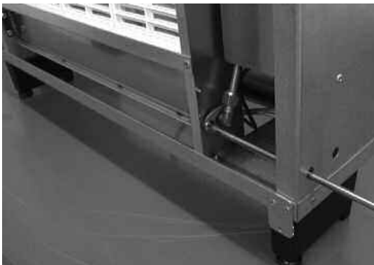
Fig. 11 Injector fixing bracket removal
