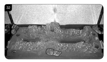
7.19 Place Log D on the left hand side of the burner. There is a hole on the underside of Log D which fits over the raised stud on the left of the burner. The back of the log should rest flat against the back panel, see Diagram 33.
