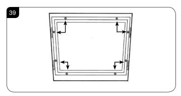
8.3 Replace ALL of the securing screws ensuring that a screw is present in all fixing slots.
