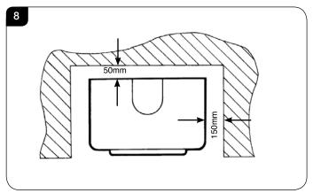
7.4 In a non-combustible recess be careful to allow enough clearance at the sides and rear of the appliance to perform spillage tests and reach the controls.
