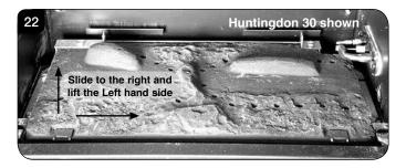
5.4 Slide the burner back to the left and out of its location.
