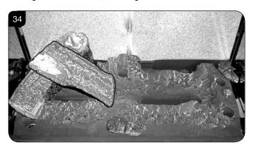
7.21 Place Log C on the right hand side of the burner. There is a hole on the underside of Log C which fits over the raised stud on the right of the burner. The back of the log should rest flush against the back panel, see Diagram 35.
