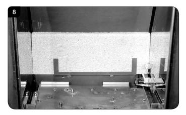
4.6 Replace all parts in reverse order ensuring the cutouts in the rear of the lower panel fit over the screws on the back of the firebox, see Diagram 9.
