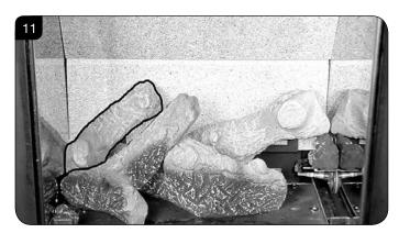
8.7 Place the pointed bottom of log D into the corner of the burner tray and rest on the location stud on log B, see Diagram 12.
