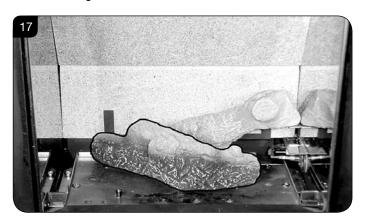
7.4 Place Log E onto the stud and behind the tag on the left hand side of the burner tray.Rest against Log B, see Diagram 18.
