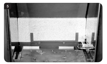
3.6 Replace all parts in reverse order ensuring the cutouts in the rear of the lower panel fit over the screws on the back of the firebox, see Diagram 6.
