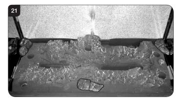
6.13 Place Log D on the left hand side of the burner. There is a hole on the underside of Log D which fits over the raised stud on the left of the burner. The back of the log should rest flat against the back panel, see Diagram 22.
