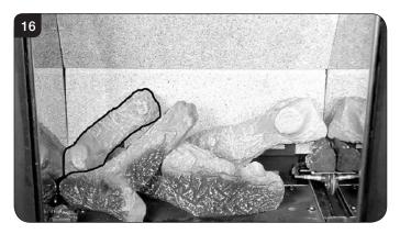
6.7 Place the pointed bottom of log D into the corner of the burner tray and rest on the location stud on log B see Diagram 17.
