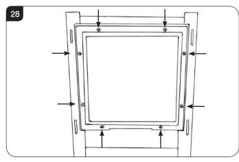
6.20 Ensure that the rope seal on the back of the door is intact, locate the door on the 4 slots and secure to the firebox, see Diagram 29.
