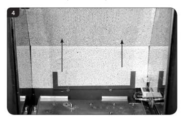
3.5 Slide the lower rear liner up and out of the lower bracket, see Diagram 5.
