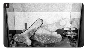
7.6 Place the small Ember at the front left of the firebox, against the rear of the log support bracket to obscure the reflection of the burner screw.
