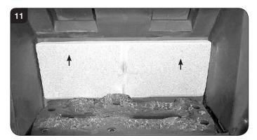
3.21 With the liners and baffle removed the firebox is clear for cleaning and maintenance, see Diagram 12.
