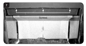
3.11 The baffle can now be removed through the front of the appliance.
