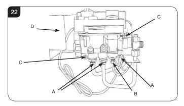
9.6 Reassemble the interruptor block and leads and secure the thermocouple connection in the rear of the gas control. (Do not overtighten).
