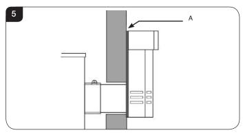
Feed the flue through the wall, making sure it runs 3.26 smoothly.
