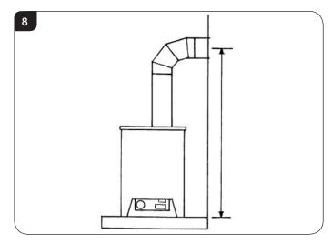
TAKE CARE TO MARK OUT THE FLUE CORRECTLY. IT 3 39 IS DIFFICULT TO MOVE AFTER INSTALLATION.
