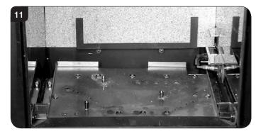
6.2 Place Log A on the higher rear bracket and push up against the back panel, see Diagram 12.
