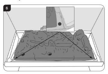
3.4 Slide the burner unit to the right, pull slightly forward and lift from the back. Carefully remove through the front of the appliance. Place carefully to one side.
