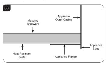
The subframe for the decorative front can now be fitted by following the instructions supplied with the Front. NOTE: THE SUBFRAME MUST SIT FLUSH TO THE WALL LEVEL WITH THE APPLIANCE FLANGE.
