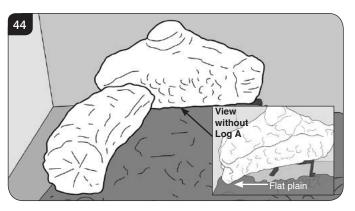
11.5 Place Log G on top of Log A. There is a hole on the underside of Log G which fits over the raised stud on Log A to secure in place. The end of the log sits on the raised section of the burner tray, see Diagram 45.
