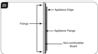
6a.11 Fit non-combustible board to the board around the appliance, see Diagram 21. Ensure distances to combustibles are observed, see Diagram 14.
