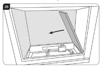
12.7 To remove the Left Hand liner first tilt inwards towards the centre of the firebox before lifting up and pulling out through the front of the firebox, see Diagram 29.
