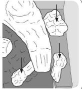
11.11 Lay Embaglow over the small ports in the base of the burner tray. This will create a glowing effect when the appliance is lit, see Diagram 51.
