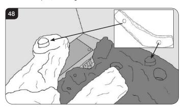
11.9 Log M should rest on the flat plain behind the stud for the Log arrangement to be complete, see Diagram 49.
