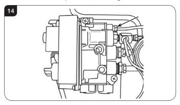
5.9 Remove the pipe and the injector drops out from the burner.
