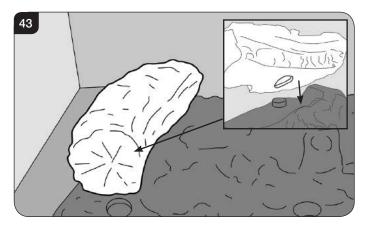
11.4 Place Log L behind the Log A on the flat plain and locate the rear of the log on the metal bracket. The log should rest between the lip of the bracket and the rear liner, see Diagram 44.
