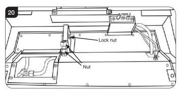
The injector can now be replaced.
