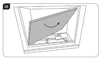
10.7 To fit the Right Hand liner insert through the front of the appliance tilting the top inwards towards the centre of the firebox before lowering into position, see Diagram 39.
