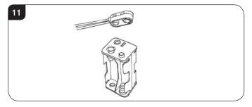
5.3 Correctly position the four new AA size batteries and re-assemble the battery holder as shown, see Diagram 12.
