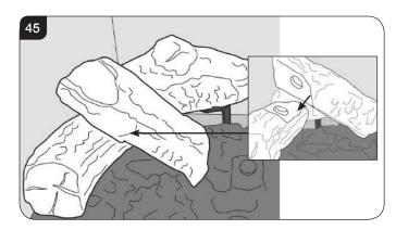
11.6 Place Log H on the centre of the burner tray. There is a raised stud in the fuel bed which securely locates the log in place. The right hand side rests on the raised section at the end of the air cutout, see Diagram 46.
