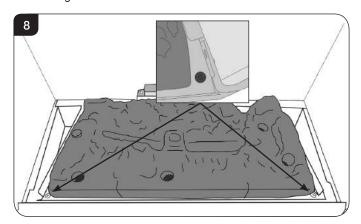
4.7 Slide the burner unit to the right, pull slightly forward and lift from the back. Carefully remove through the front of the appliance. Place carefully to one side.
