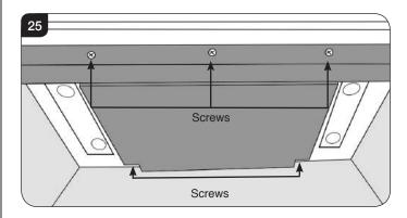
12.5 The baffle can now be removed by lowering the front edge and pulling forward through the front of the appliance. TAKE CARE NOT TO DAMAGE THE SIDE PANELS
