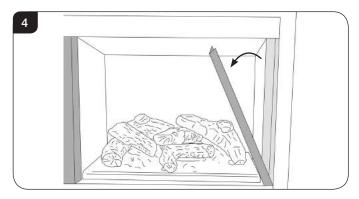
4.3 Lift out the bottom slotted trim, see Diagram 5.
