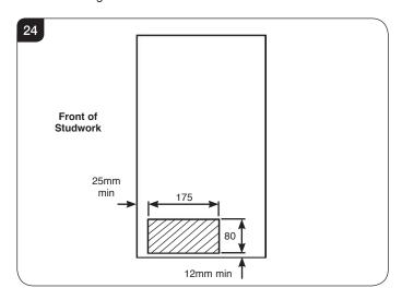
6b.4 Line the aperture for the appliance with 12mm thick non-combustible material as shown. Non-combustible board used to protect the studwork can line the aperture inside the 50mm clearance distance, see Diagram 25.
