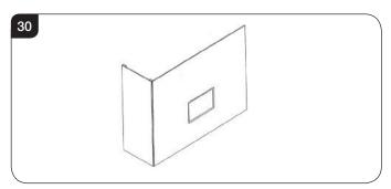
6.8 A removable access hatch must be left in the side of the chimney breast for future servicing and inspection of the appliance.
