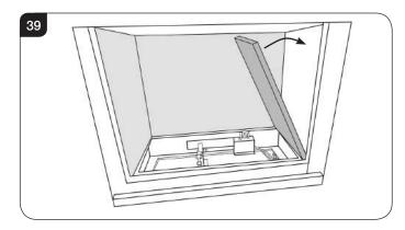
10.8 To fit the Left Hand liner insert through the front of the appliance tilting the top inwards towards the centre of the firebox before lowering into position, see Diagram 36.
