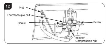
5.4 The pilot unit can now be removed and the pilot components can now be individually removed and replaced.
