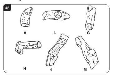
11.3 Place log A on the left hand front of the burner. The log will fit over the raised stud and into the groove in the burner tray, see Diagram 43.
