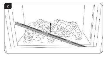
2.3 Remove the 2 screws at the base of the glass frame, see Diagram 3.
