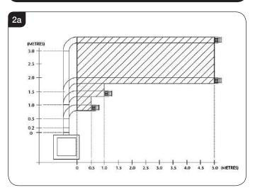
Start of bend to centre line of horizontal flue 170mm. Centre line of vertical flue to end of bend 220mm.
