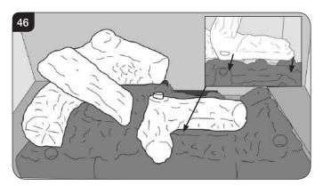
11.7 Rest Log J on the raised stud on Log H. The rear of the effect should rest on the metal bracket at the back of the burner tray, see Diagram 47.
