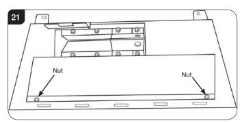
11.4 Remove the 2 fixing nuts and slide the plate off the venturi, see Diagram 22, the Aeration Plate can now be replaced.
