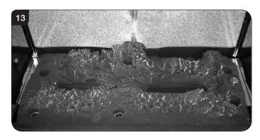
7.12 There are 3 embers. Place 2 embers in the back corners of the burner, resting in the cut outs, see Diagram 14. Place the last ember loosely at the front of the fuel bed to cover the hole in the centre.
