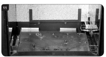
6.2 Place Log A on the higher rear bracket and push up against the back panel, see Diagram 12.
