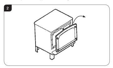
5.2 Remove the glass frame by undoing the fixing screws and lifting clear, see Diagram 3. Take care to support the glass window panel when removing the screws.
