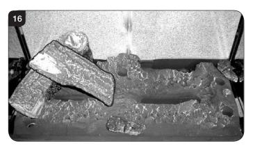
7.15 Place Log C on the right hand side of the burner. There is a hole on the underside of Log C which fits over the raised stud on the right of the burner. The back of the log should rest flush against the back panel, see Diagram 17.
