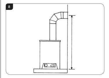
3.39 TAKE CARE TO MARK OUT THE FLUE CORRECTLY. IT IS DIFFICULT TO MOVE AFTER INSTALLATION.
