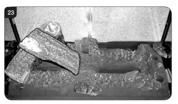
6.15 Place Log C on the right hand side of the burner. There is a hole on the underside of Log C which fits over the raised stud on the right of the burner. The back of the log should rest flush against the back panel, see Diagram 24.
