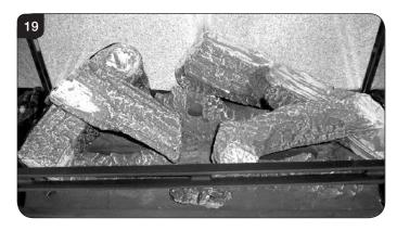
7.18 Once the logs are in place sparingly spread an amount of the Embaglow fibres provided on the sections highlighted, see Diagram 20.
