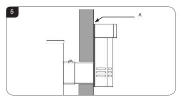
3.26 Feed the flue through the wall, making sure it runs smoothly.
