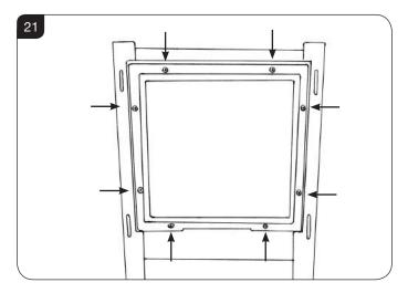
7.20 Ensure that the rope seal on the back of the door is intact, locate the door on the 4 slots and secure to the firebox, see Diagram 22.
