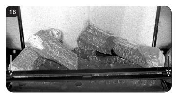
7.16 Place Log A across Log C. There is a hole on the underside of Log A which fits over the raised stud on Log C to secure in place. The small cut out on the left side of the log rests onto the log guard, see Diagram 19.
