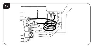
8.10 Remove the pipe and the injector drops out from the burner.
