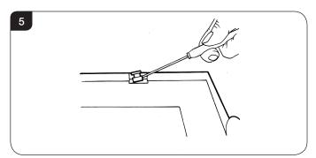
4.2 Lift the glass clear from the lock bracket at the top of the frame and slide out.
