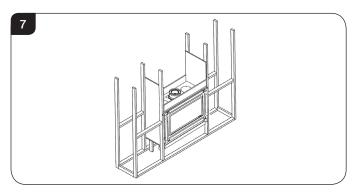
4.8 Attach the 4 x frame fixing brackets to the appliance, see Diagram 8.
