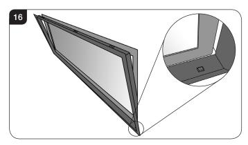
5.16 Push the top into place within the opening, taking care not to damage the frame or the wall finish, see Diagram 17.
