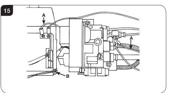
7.8 Disconnect the battery extension lead, Diagram 15, B.
