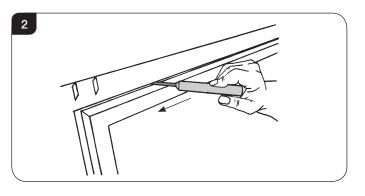
To completely remove the glass front:
