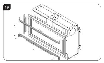
6.2 This now determines the width of your two vertical studwork supports. The kit has been designed so that non-combustible board can be taken right up to the edge of the four brackets, see Diagrams 20 & 21.
