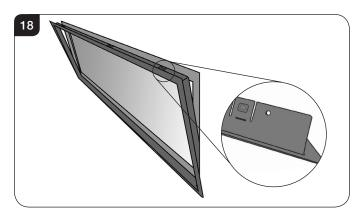
5.19 If the Edge+ is too loose the tabs can be bent up to gain better purchase on the edge of the appliance box.If the Edge+ is too tight the tabs can be bent downwards to give more clearance.
