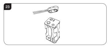
7.3 Correctly position the four new AA size batteries and re-assemble the battery holder as shown, see Diagram 24.
