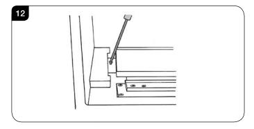
6.4 Slide the burner fully to the left and lift the right side clear of the pilot, see Diagram 13.
