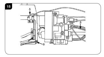
7.8 Disconnect the battery extension lead, Diagram 18, B.
