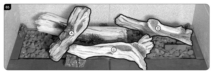
13.4 Log H sits across the right hand and front liners, with the charred side facing out, see Diagram 66. Log L sits across the left hand and front liners, with the charring facing left, see Diagram 66. Once all the logs are in place the remaining 2 small embers can be positioned on the front liner.
