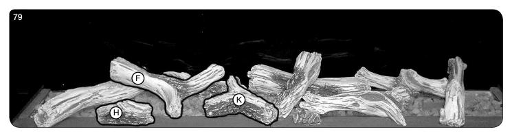
13.24 1 x Log L locates in the rear left corner and 1 x Log H sits on the front liner panel, see Diagram 80.
