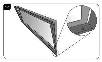
Push the top into place within the opening, taking care not to damage the frame or the wall finish, see Diagram 18.
