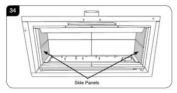
NOTE: THE HORIZONTAL CHAMFERS MUST ALIGN ON THE REAR AND SIDE PIECES.
