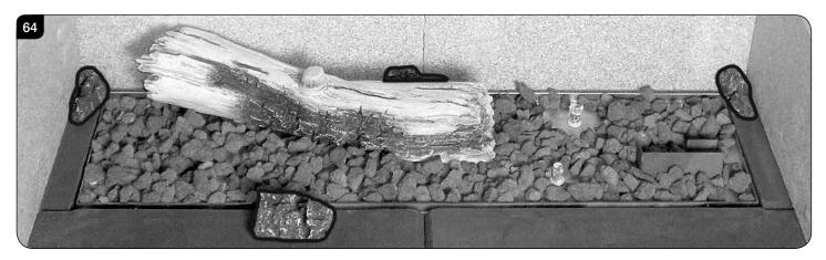
13.3 Log D is positioned in the rear right hand side of the burner tray, and rests on the Pilot Shield, see Diagram 65. **Ensure the log rests on the burner tray and not lava rocks.**
