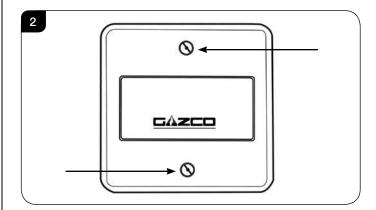
3.2 Unclip the battery holder from the wall plate and remove the old batteries.
