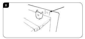
4.10 Fix foam seal to the rear of the outer flange of the appliance, see Diagram 9.
