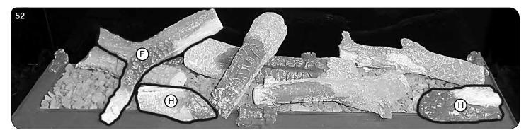
12.14 Log G sits on the left hand and front liner. Once in place the final ember can be positioned to the right of Log C, see Diagram 53.
