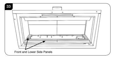
9.7 Slide the 2 side panels up to the rear panel, see Diagram 34.
