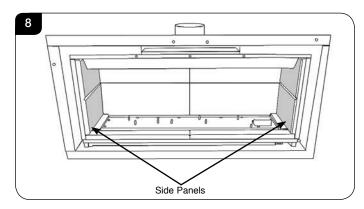
NOTE: THE HORIZONTAL CHAMFERS MUST ALIGN ON THE REAR AND SIDE PIECES.
