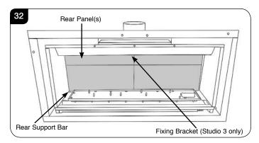
If installing the panels on a Studio 3 model replace the L shaped fixing bracket at the top rear of the firebox to hold the two rear liners in place.
