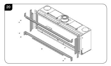
This now determines the width of your two vertical studwork supports. The kit has been designed so that non-combustible board can be taken right up to the edge of the four brackets, see Diagrams 21 & 22.
