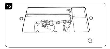
7.5 Remove the six screws securing the control assembly, see Diagram 16.
