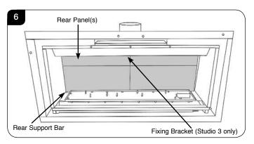
If installing the panels on a Studio 3 model replace the L shaped fixing bracket at the top rear of the firebox to hold the two rear liners in place.
