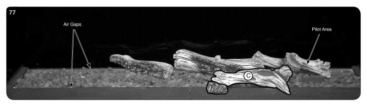
13.22 Log J is positioned on the front lower liner panel with the rear resting on the pin at the rear of the fuel bed, see Diagram 78. Log A located on the stud on Log B and the front edge on the edge of the burner tray, see Diagram 78. The rear of Log M rests on the right hand edge of Log D and place the front on the front lower liner panel, see Diagram 78.
