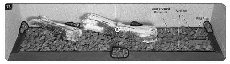
13.12 Log D is positioned on the right pin to the rear of the burner tray, and rests on the Pilot Shield, see Diagram 77.
