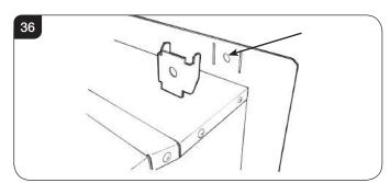
7.17 Attach the foam seal around the rear of the flange, see Diagram 37.
