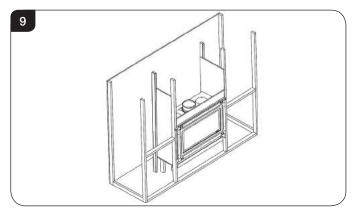
4.9 Attach the 4 frame fixing brackets to the appliance, see Diagram 10.
