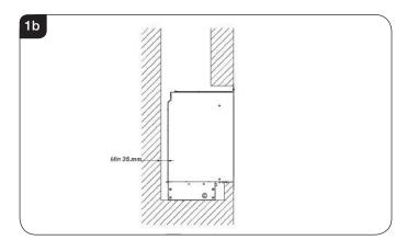
5.4 **DO NOT** install onto a combustible wall; all combustible materials must be removed from the area shown in Diagram 1c.
