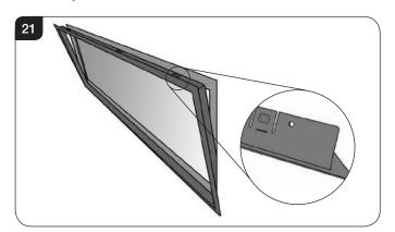
5.21 If the Edge+ is too loose the tabs can be bent up to gain better purchase on the edge of the appliance box.If the Edge+ is too tight the tabs can be bent downwards to give more clearance.
