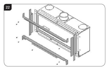
6.2 This now determines the width of your two vertical studwork supports. The kit has been designed so that non-combustible board can be taken right up to the edge of the four brackets, see Diagrams 23 & 24.
