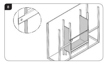
4.8 Fit the support bar into the studwork at the correct height, see Diagram 9.
