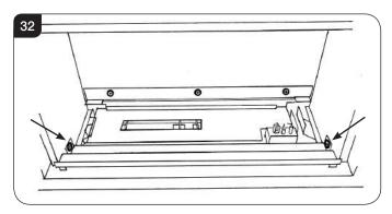
7.11 Remove the three screws retaining the rear back panel.
