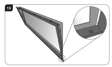
5.18 Push the top into place within the opening, taking care not to damage the frame or the wall finish, see Diagram 20.
