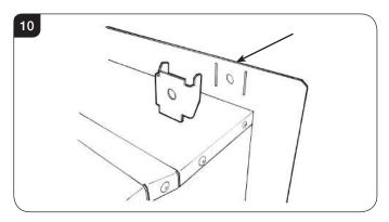
4.10 Fix foam seal to the outer flange of the appliance, see Diagram 11.
