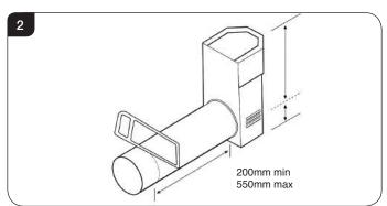
Terminal dimensions: 395 x 200 x 200 mm (H x W x D) Guard supplied Cut to length as required on site, see Diagram 2.
