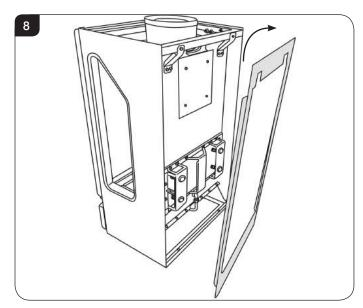
3.17 Tighten the 4 loose screws (Diagram 7, Arrow B) and replace the top 2 screws (Diagram 7, Arrow A).
