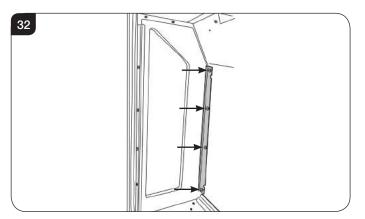
13.3 Replace the glass and gasket, ensuring that the printed side is facing outwards.
