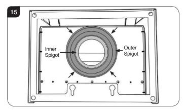
4.5 Swap the inner and outer flue spigots **<u>only</u>** with the inner and outer blanking plates on the rear of the appliance, see Diagram 16.
