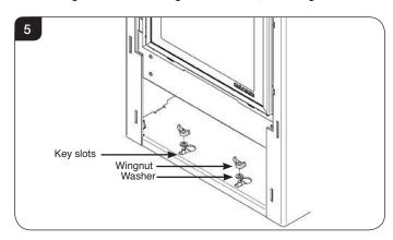
3.8 Place the 2 large washers over the studs and fix with 2 wingnuts, see Diagram 5.
