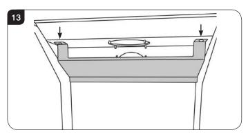
Note: When replacing the Rear Baffle ensure that the tab locates behind the rear panel slot, see Diagram 14.
