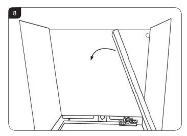
Support the rear panel when handling the last side and remove carefully.
