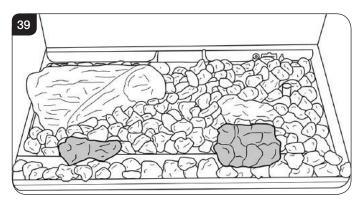
9.5 Log B is positioned on the right hand locating pin, and rests against the back liner, see Diagram 40.
