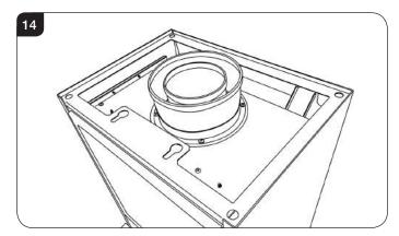
4.4 Remove the 8 screws securing the inner & outer spigots, see Diagram 15.
