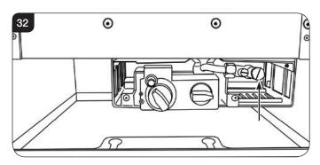
7.2 Connect a suitable pressure gauge to the test point located on the inlet fitting and turn the gas supply on. Light the appliance and check all gas joints for possible leaks. Turn the appliance to maximum and check that the supply pressure is as stated on the databadge. Turn the gas off and replace the test point screw, turn the gas on and check the test point for leaks.
