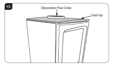
4.3 The cast top plate lifts off to give access to the inner and outer flue spigots, see Diagram 14.
