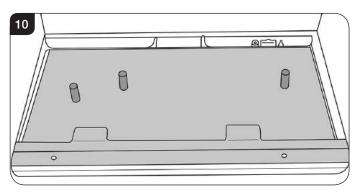
7.2 Place Log A in position on the 2 locating pins, see Diagram 11.
