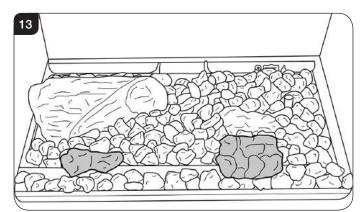
7.5 Log B is positioned on the right hand locating pin, and rests against the back liner, see Diagram 14.
