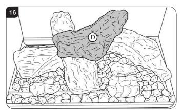
7.8 Spread a liberal amount of the Embaglow fibres provided on the sections highlighted, see Diagram 17.
