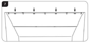
4.2 The baffle can now be removed through the front of the appliance.
