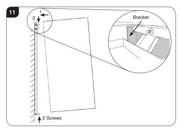
NOTE: The top rear edge of the appliance must locate between the back lip of the wall mounting bracket and the raised supports, see Diagram 12.
