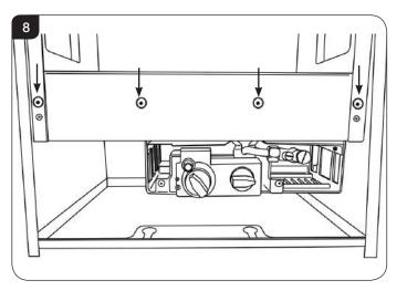
5.6 The frame can be removed by lifting the hooks clear of the slots from the bottom of the frame and lifting away from the appliance, see Diagram 9.
