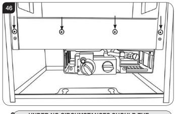
UNDER NO CIRCUMSTANCES SHOULD THE APPLIANCE BE USED IF ANY OF THE GLASS FRAME RETAINING SCREWS ARE LOOSE OR MISSING. 10.3 Fit the front by inserting the hooks on the back of the frame into the slots on the front of the appliance, see Diagram 47.
