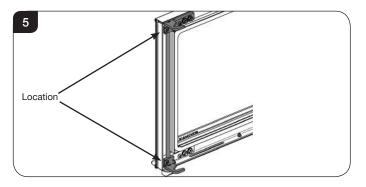
5a.3 The top and bottom catches will need to be adjusted separately and in the same manner. The catch block can move in two directions, see Diagram 6, 7 & 8.
