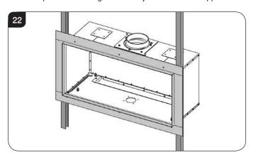
4.3 Fit non combustible board to studwork/frame/masonry and leave enough room for the final skim of heat resistant plaster.
