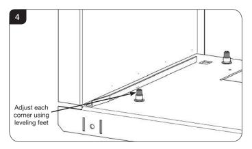
Wind the set screws down to the desired position in each corner.
