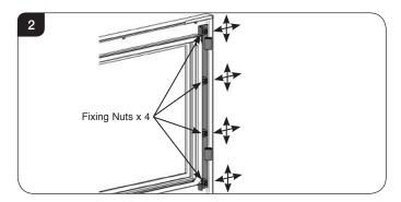
4a.5 Loosening the Door Hinge Assembly allows for fine vertical and horizontal adjustment of the door position. This may require a trial and error approach to find the correct position. Ensure the door is horizontal before tightening the fixing nuts.
