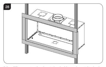
5.3 When constructing the studwork chimney breast the depth of the Cool Wall flange will vary depending on the model of Studio.
