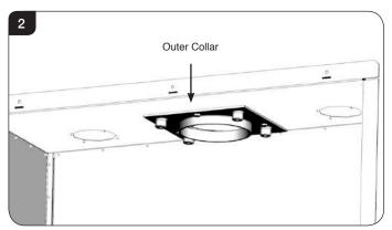
Using a 13 A/F Spanner remove the 3 bolts and remove outer collar.
