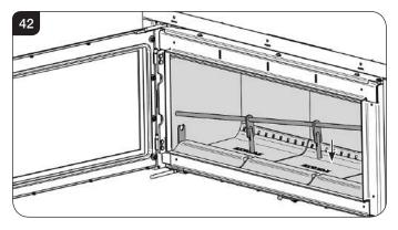
Slide the Log Guard across so both ends locate evenly in the holes in the side bricks, see Diagram 43.
