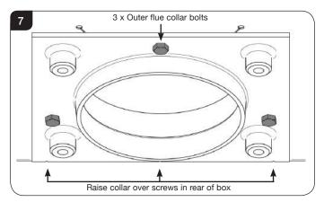
2.9 To ensure the outer collar is central, and **to avoid cross threading of the bolts** during actual installation, feed the
