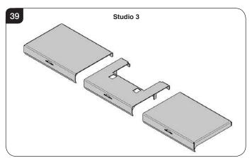
The Studio 3 baffle comes in three sections. To fit the baffle system the baffles must be placed in the firebox in the following order:
