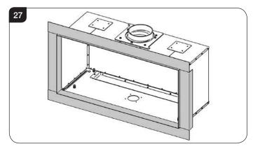
5.2 The frame determines the width of the two vertical studwork supports. The kit has been designed so that noncombustible board can be taken right up to the edge of the frame, see Diagram 28.
