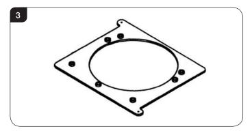
2.3 If the optional fan is to be fitted, remove the fan cover in the base of the outer case. This cannot be removed after the outer case has been installed. Full instructions are included with the fan (PM379).
