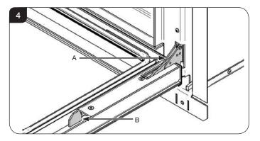
4b.3 Open and close the door a few times to work the grease into the hinge to return it to smooth operation.
