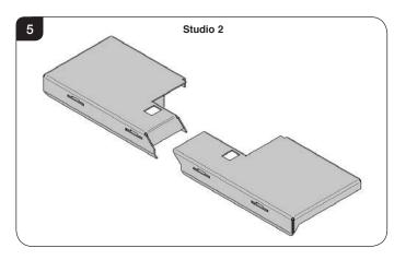
The Studio 2 baffle comes in two sections. To remove the baffle system first disengage the left hand side. The method of removal is the same for both sections.
