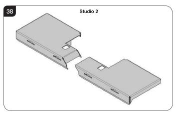
The Studio 2 baffle comes in two sections. Fit the right hand side baffle first. The method is the same for both sections.
