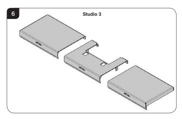
The Studio 3 baffle comes in three sections. To remove the baffle system the baffles must be taken out in the following order:
