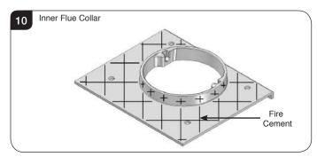
2.14 Fit the inner flue collar using the 4 bolts ensuring the 2 longer bolts are at the front and recessed into the Flue Collar, see Diagram 11.
