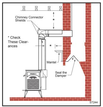
Fig. 7 Chimney connector enters chimney above the firep. lace.
