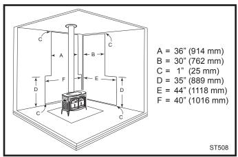
**Fig. 21** Parallel installation, vertical chimney connector, two wall shields. Reduced clearances for both rear and side walls. Wall shields may meet at corner if desired. Shielding for connector is centered behind connector.
