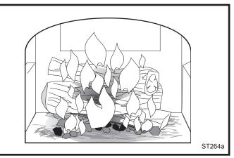
**Fig. 41** Add full size logs when the ember bed is 3" (75mm) deep.
