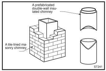
Fig. 2 Standard chimney types.
