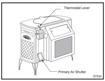
Fig. 43 The primary air shutter must move freely.
