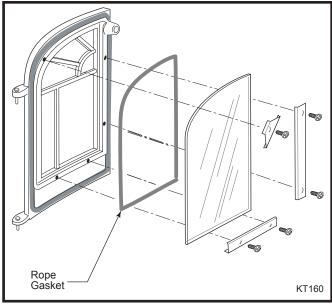
Fig. 42 Door glass installation.
