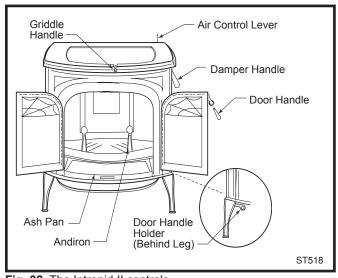
Fig. 32 The Intrepid II controls.
