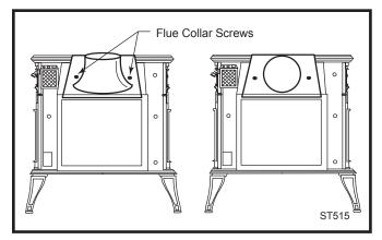
Fig. 30 Reversing the flue collar.
