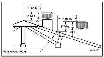
Fig. 3 The 2'-3'-10' Chimney Rule.
