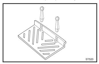
Fig. 35 Remove the andirons for front loading.
