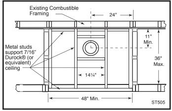
Fig. 19 Reflected ceiling plan.
