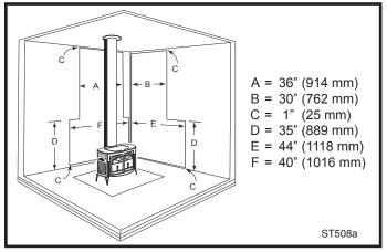
**Fig. 24** Parallel installation, vertical chimney connector, with stove, connector and wall shields. Maximum reduction for rear and side walls. Wall shields may meet at corner. A heat shield 24" (610mm) in diameter suspended 1" (25mm) below the ceiling must surround the chimney.
