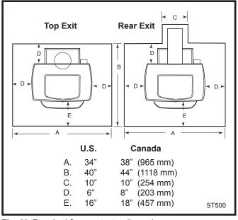
Fig. 11 Required floor protector dimensions.
