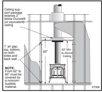
**Fig. 20** Front view: 65" minimum clearance form hearth to combustibles on front face. Combustible facing may overlap metal studs by only 1". It should not extend below the height of the noncombustible ceiling.
