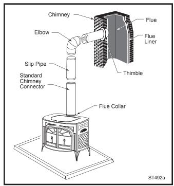
Fig. 6 Chimney connection in a freestanding installation.
