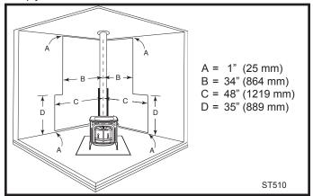
**Fig. 23** Corner installation, vertical chimney connector, with rear, stove, connector and wall shields. Wall shields **MUST** meet at corner. Connector heat shield extends 28" (710mm) above flue collar. A 24" (610mm) diameter ceiling heat shield must surround the chimney and be suspended 1" (25mm) from ceiling.
