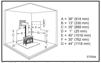
**Fig. 25** Parallel installation with rear wall pass-through, with stove, connector and wall shields. Wall shields may meet at corner. Connector heat shield extends 28" (710mm) above flue collar, or below elbow, whichever is less. Wall pass-through must comply with codes.
