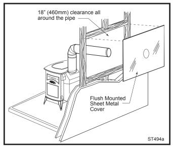
Fig. 10 An approved wall pass-through for Canada.
