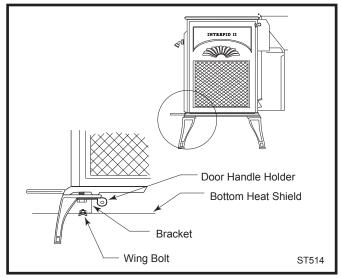
Fig. 29 Handle holder and heat shield positions.
