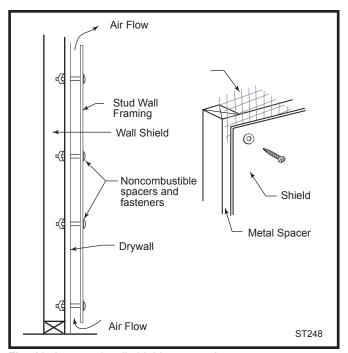
Fig. 13 Approved wall shield construction.
