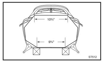
Fig. 28 Attach bottom heat shield.
