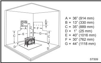
**Fig. 22** Parallel installations with rear wall pass-through, two wall shields. Reduced clearances for both rear and side walls. Wall shields may meet at corner if desired. Shielding for connector is centered behind connector. Wall pass-through must comply with codes.
