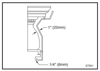
Fig. 14 A custom-formed mantel shield.
