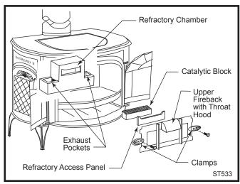
Fig. 46 Removing the catalytic element.
