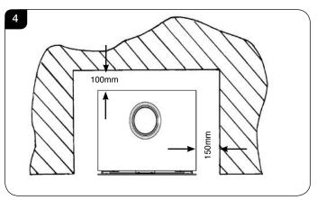
5.10 The above dimensions provide adequate clearance to combustible materials. It may be necessary to add additional clearance so that spillage tests can be performed when necessary.
