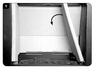
4.10 To remove the Right Hand liner first tilt inwards towards the centre of the firebox before lifting up and pulling out through the front of the firebox, see Diagram 10.
