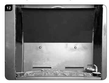
4.13 To replace the liners liner and baffle reverse these procedures.
