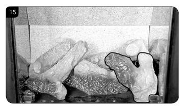
8.8 Use some of the Embaglow provided and cover the ports in the burner tray with a liberal amount of fibres. Use a small piece in front of the log on the left hand side and a long strip in front of log B, see Diagram 16.
