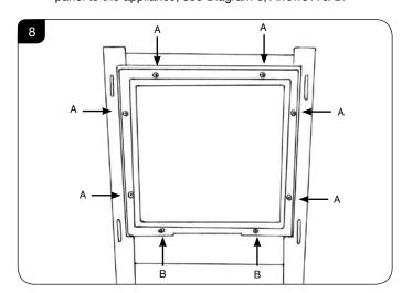
Take care to support the glass when removing the screws.
