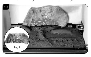
8.12 Place the second log into the left hand groove on the burner tray, see Diagram 20.
