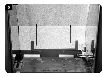
4.5 Slide the lower rear liner up and out of the lower bracket, see Diagram 6.
