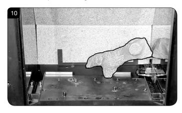
8.3 Place Log B over the two middle studs on the burner tray, see Diagram 11.
