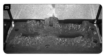
8.18 There are 3 embers. Place 2 embers in the back corners of the burner, resting in the cut outs, see Diagram 26. Place the last ember loosely at the front of the fuel bed to cover the hole in the centre.
