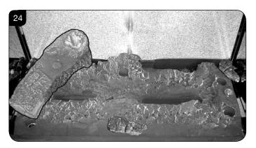
7.20 Place Log B on top of Log D. There is a hole on the underside of Log B which fits over the raised stud on Log D to secure in place. The right hand side of the log rests in the groove in the burner, see Diagram 25.
