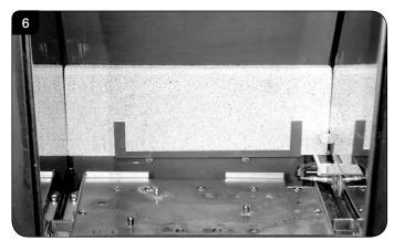
4.6 Replace all parts in reverse order ensuring the cutouts in the rear of the lower panel fit over the screws on the back of the firebox, see Diagram 7.
