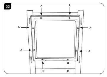
9.2 Replace ALL of the glass frame securing screws ensuring that a screw is present in all fixing slots.
