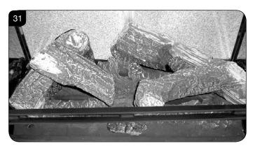
8.24 Once the logs are in place use some of the Embaglow wire wool provided and cover the ports in the burner tray with a liberal amount of fibres, in the highlighted areas shown in Diagram 32.
