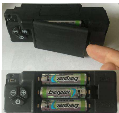
Batteries in the Gas Valve Controller Mounted at the front of the stove
