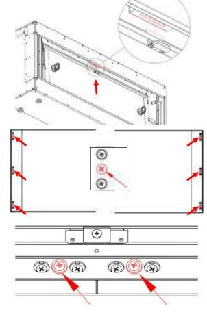
Trim Installation **3.5.2** Once the non-combustible board has been fixed to the studding, the trim can now be fitted to complete the installation.
