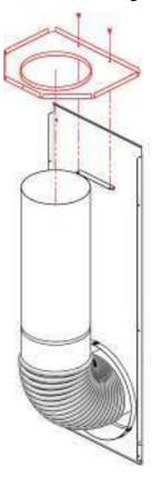
Now slide the terminal cover into position, ensuring the vertical flue alignment bracket is located **between the two guide brackets** on the inside of the terminal body.
